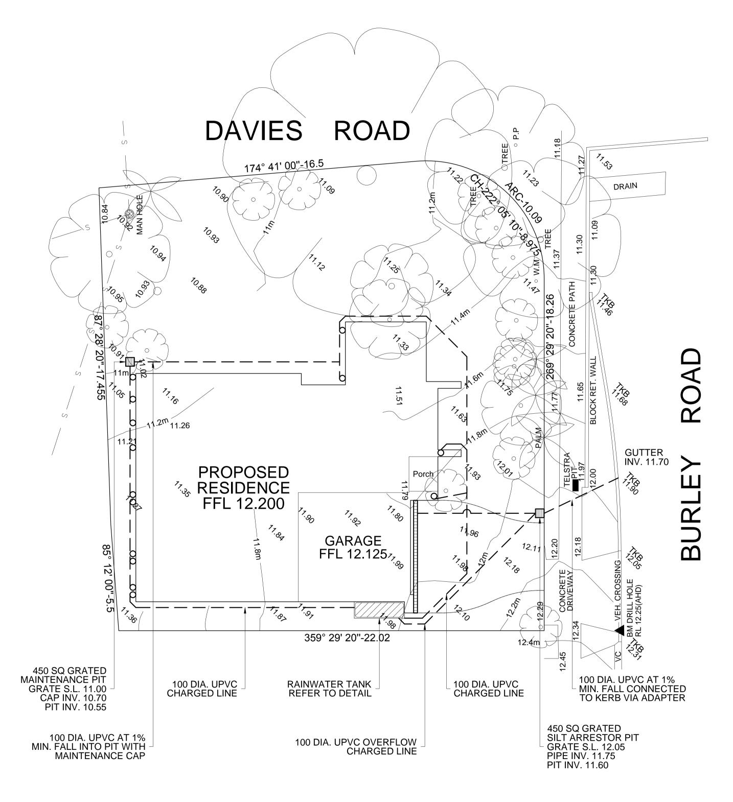
**CALCULATIONS** = 531.0m<sup>2</sup> SITE AREA IMPERVIOUS AREA = 222.0m<sup>2</sup> SINCE 42% < 75% NO DETENTION REQUIRED
